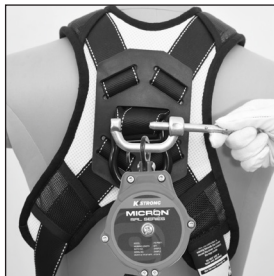
Open connector by pushing the locking lever and push button at the end simultaneously.
